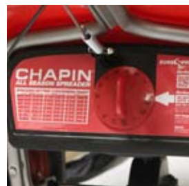
Gate setting dial with reference chart Check the reference chart, set the dial and the gate will open as much as needed.
