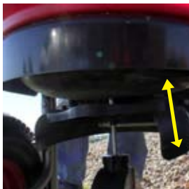
Edge Control Control spread pattern when near sidewalks
