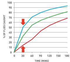
Mean catch of the Genus® Cobra™ 45 Watt translucent trap compared with two leading competitor units over a three hour period.
