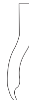
Fill Tube Spout Aire Gap (All) Flex Gap (D4 only) P/N 7630041-A Flex Gap (Single Prod Only) P/N 7630041-F
