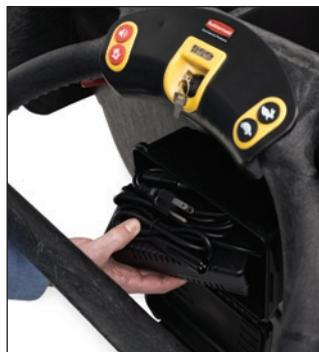
On-board storage for the external charger allows battery to be recharged at any standard 120v wall outlet.
