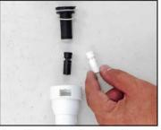
A unit can be changed from a 3.8 LPM unit to a 15.2 LPM unit with a switch of the venturi.
