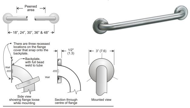
Concealed mounting screws, using snap flange, on "SP & NP" codes
