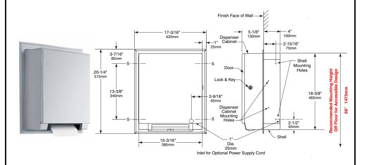
Rough Wall Opening 16" (405mm) wide 18-7/8" (480mm) high 4" (102mm) minimum recessed depth
