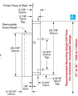
Rough Wall Opening 15-7/8" (405mm) wide 26-1/4" (665mm) high 4" (100mm) minimum recessed depth
