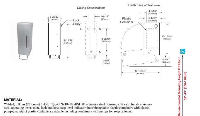
Welded, 0.8mm (22 gauge) 1.4301, Typ CrNi 18/10, AISI 304 stainless steel housing with satin finish; stainless steel operating lever; metal lock and key; soap level indicator; interchangeable plastic containers with plastic pumps; variety of plastic containers available including containers with pumps for soap or foam.
