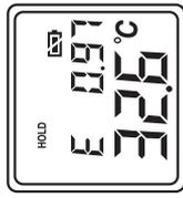
**Simply aim the thermometer at the measure target with Lens (6) and press Meas. key (8) to display the surface temperature.**
