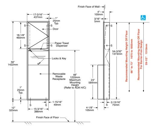
Rough Wall Opening 16" (406mm) wide 54-3/4" (1390mm) high 4" (100mm) minimum recessed depth
