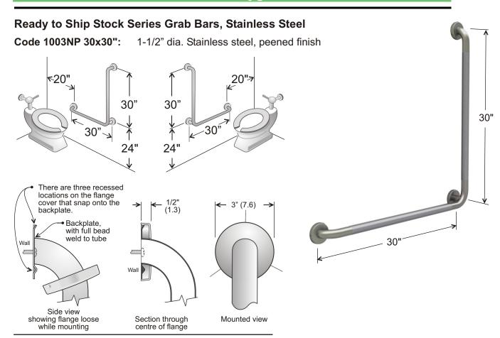
Concealed mounting screws, using snap flange, on "SP & NP" codes
