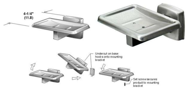
**Mounting of Product:** Screw concealed mounting system: The mounting bracket is attached to the wall with screws at the desired height. The unit is then hooked onto the bracket. When the set screw is tightened the product is firmly secured to the wall. The set screw applies pressure to an inclined surface on the bracket this provides a rattle free and integral mounting of the product. (mounting bracket and screws provided).
