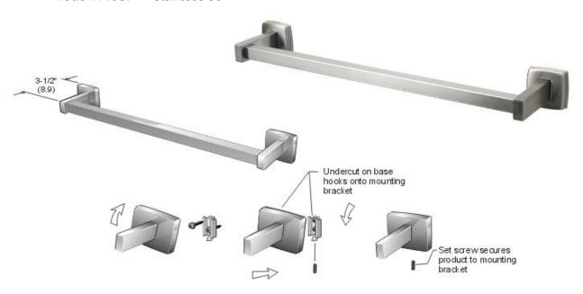
**Mounting of Product:** Screw concealed mounting system: The mounting bracket is attached to the wall with screws at the desired height. The unit is then hooked onto the bracket. When the set screw is tightened the product is firmly secured to the wall. The set screw applies pressure to an inclined surface on the bracket this provides a rattle free and integral mounting of the product. (mounting bracket and screws provided).
