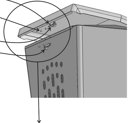
**How the lock latch appears when assembled.**
