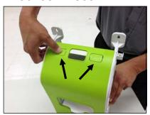
APPLICATION NOTE: The covers have knockout plugs that can be removed if desired to allow the chemical line to be routed into an F-style container.
