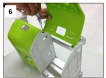
Attach add-on cover to the side panels using the 2 screws. Ensure the hinges are oriented so that screws are not visible when the cover is down. Repeat steps 4 through 6 for any additional cabinets.
