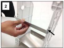
Insert the back brace into the corresponding slots on the left and right side panels so that the brace will sit flush against the wall when mounted.
