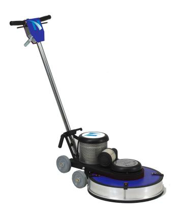
The all steel construction and and 1.5hp DC rectified motor ensure this unit can handle the toughest of jobs. The multi-grooved drive belts provide efficient power transfer. This model also features a unique filter system for dust control that is easily cleaned and changed. The NA 1520DC complies with LEED - EB EQ credit 3.7 for sustainable cleaning equipment.
