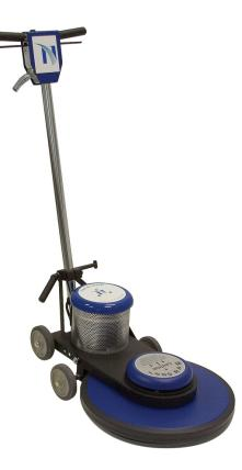
2000 RPM Burnisher Motor is 1.5 Hp DC rectified Weighs 112 lbs and is 20" wide Heavy duty steel construction throughout Belt drive system Burnishers are rugged and reliable Multi-grooved drive belts transmit the power and speed from
