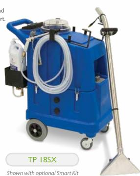
The TP 18SX is a premium extractor featuring a 130 psi pump with 1.2 gpm of water flow. The 18 gallon polyethylene tanks are designed to clean large areas and it comes complete with a 20' solution/vacuum hose and three-jet wand.
